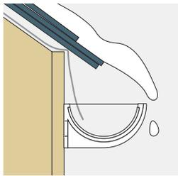
Fix brackets so as to position the gutter centrally and as close below the roof edge as possible, taking into consideration locality and roof slope finish. If there is a risk of sliding snow, adjust the bracket positions to prevent snow hitting the front of the gutter. Extra fixings, brackets and snowboards should be considered where appropriate.
