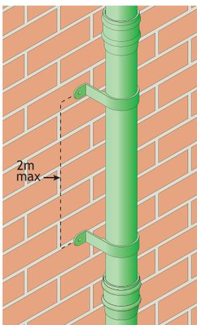
Where unearred pipework is being used it must be secured at maximum 2m centres.
