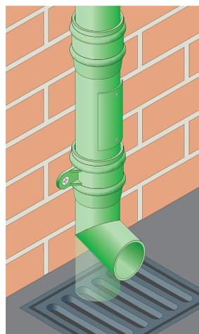
At ground level rainwater pipes can terminate with a shoe for free discharge over a gully or be directly connected into the gully.
